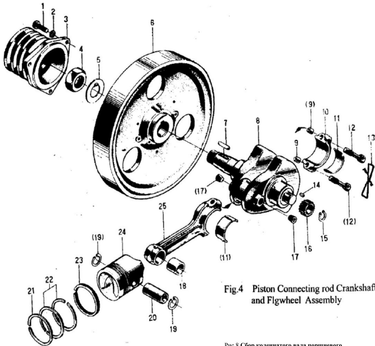
Fig.4 Piston Connecting rod Crankshaft and Flywheel Assembly
