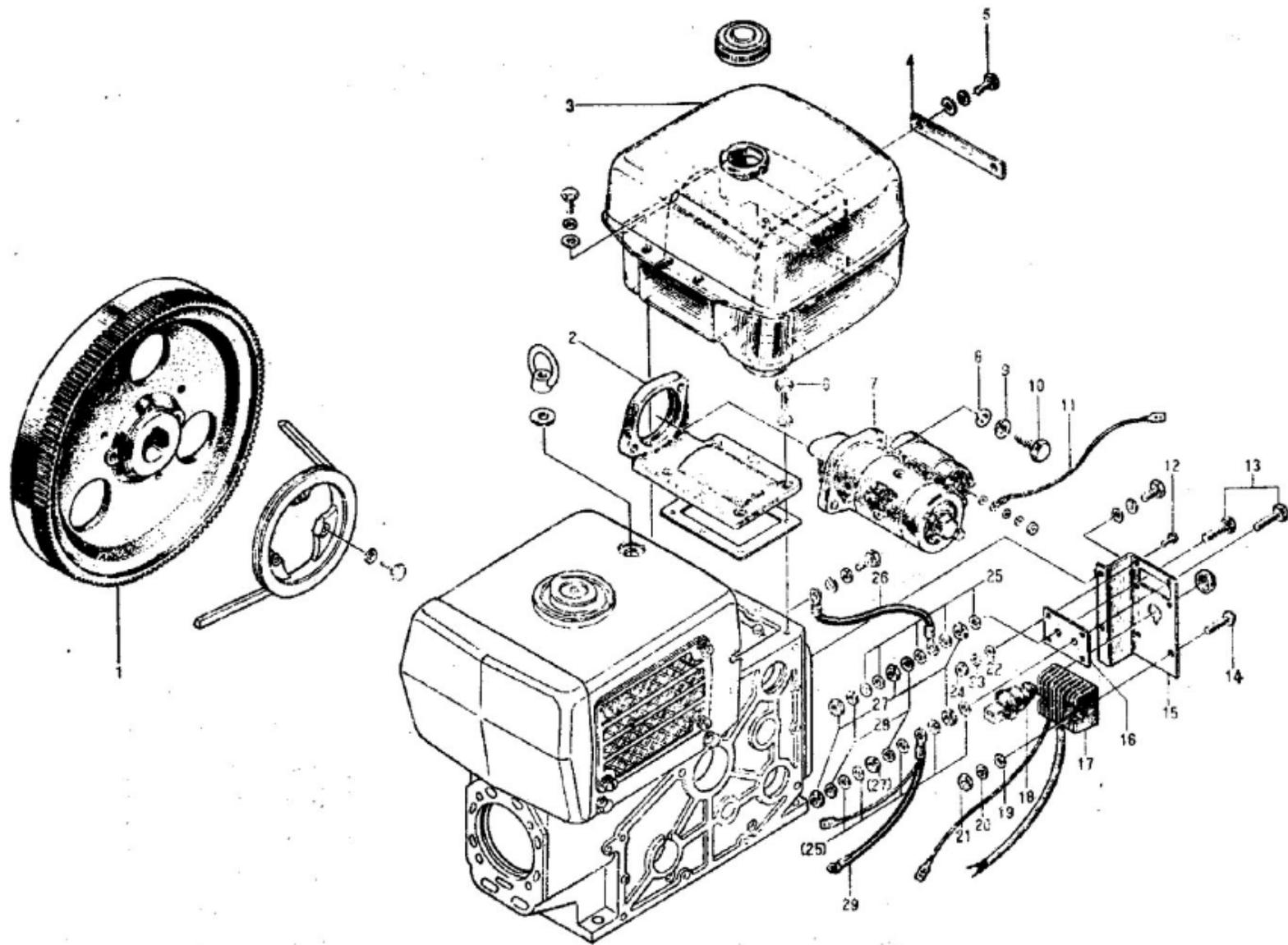
Fig. 11 Special Parts for Model S195M/S1100M Diesel Engine
