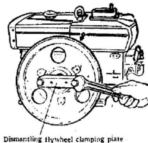
**Fig. 11 Pull out the flywheel with a puller**
