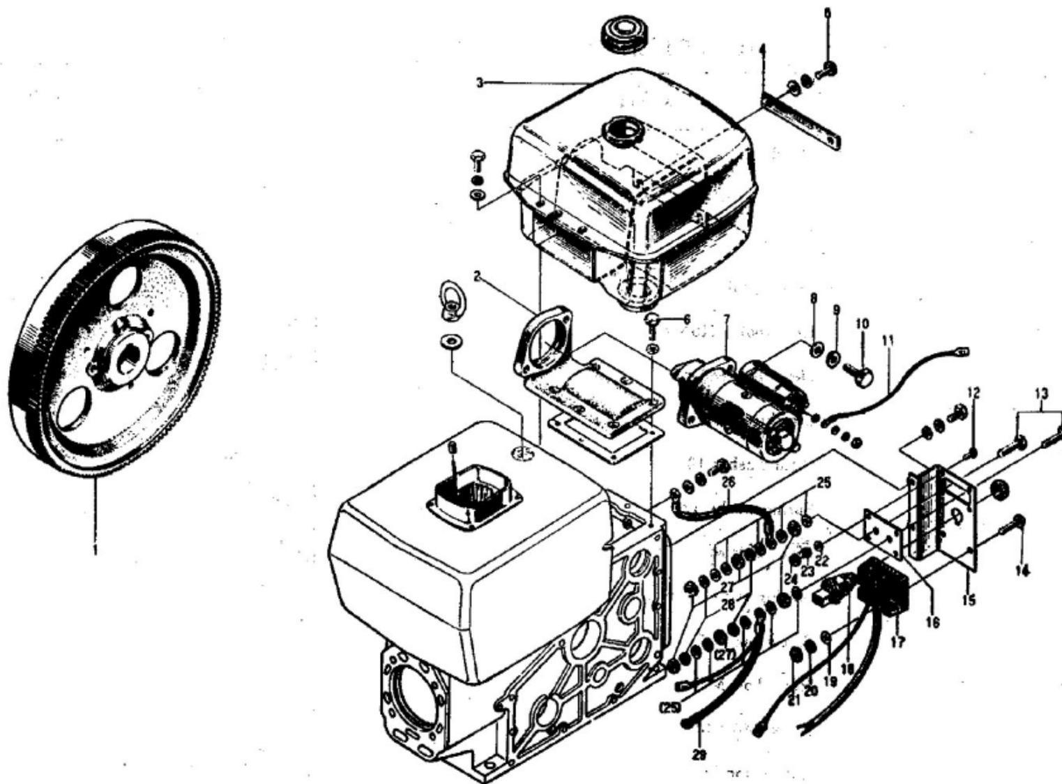
Fig. 11 Special Parts for Model S195NM/S1100NM Diesel Engine
